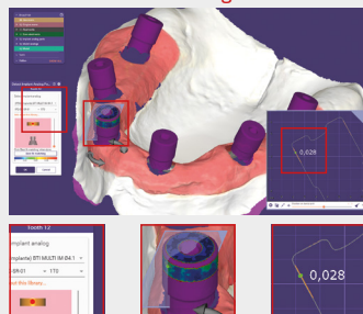
NOK. Best fit with wrong tolerance
